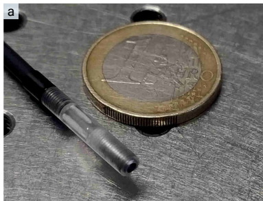
Photo of the fiber probe (a) and 3D rendering (b)
